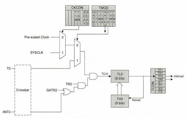
Figure 23.2. T0 Mode 2 Block Diagram
