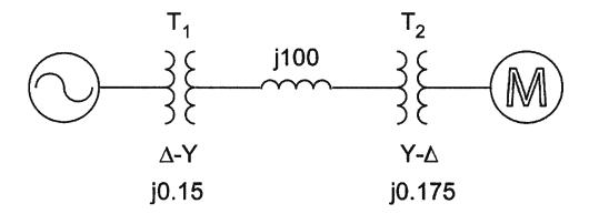
Draw the per-unit positive sequence equivalent circuit.
