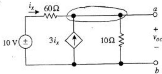
Determine the Thevenin equivalent circuit with respect to terminals *a* and *b*.
