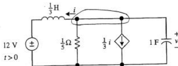
$$\begin{aligned}v(0^+) &= 3 \text{ V} \\i(0^+) &= 9 \text{ A}\end{aligned}$$
