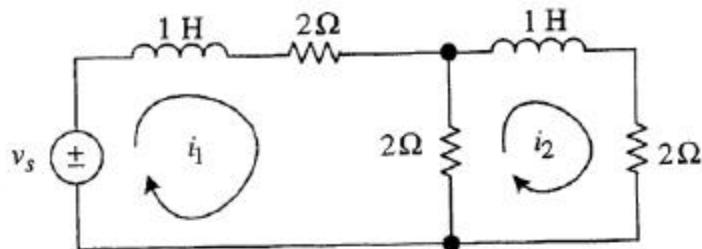
Determine the natural-response component of mesh current  $i_1$ .
