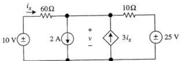
Use superposition to calculate voltage  $v$ .
