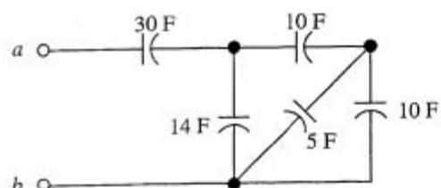
$$C_{eq} = \underline{\quad 12 \quad} \text{ F}$$
