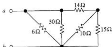
$$R_{eq} = \underline{\quad 4 \quad} \Omega$$
