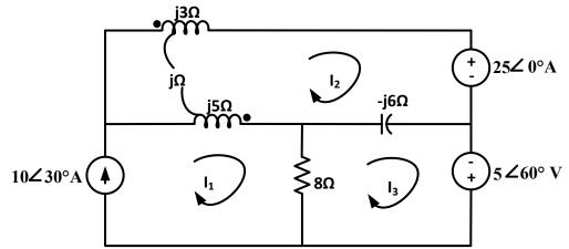
Write a set of mesh current equations in the matrix form. Do not solve. (25 pts)
