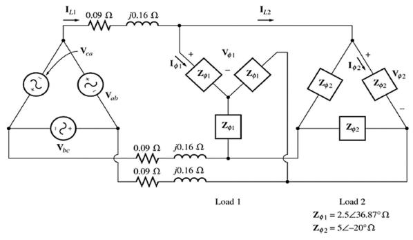
a. Draw the per-phase equivalent circuit with correct values of all components. Take phase A line-to-neutral voltage to be your angle reference. (5 points)
