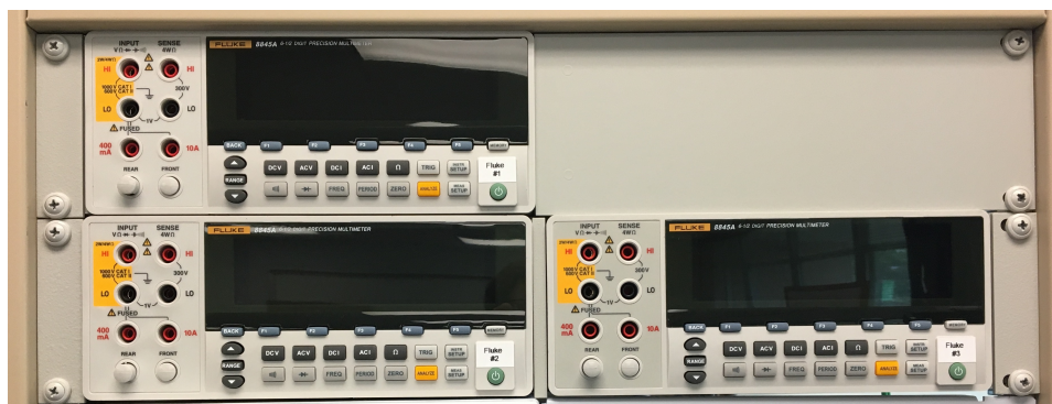
Figure 2: Rack-mounted Fluke 8845A multimeters
