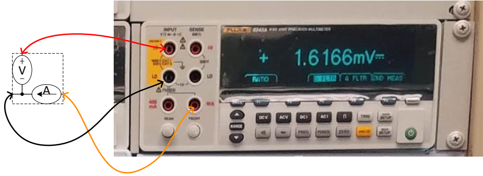
Figure 4: Mapping of Fluke 8845A terminals to schematic.
