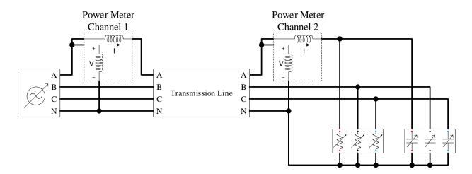
Figure 7: Experimental configuration with VAR compensation.
