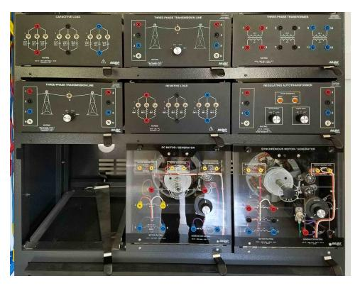
Figure 5: LabVolt equipment for low-power experiments on power distribution networks.
