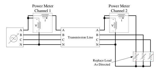
Figure 6: Configuration for experiment with a single load (swap out the resistive load box).
