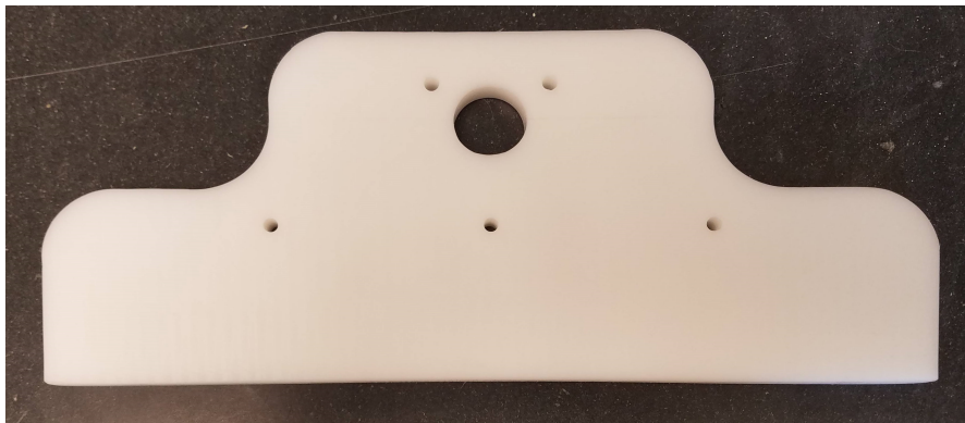
Figure 7: Plastic piece used to block the rotor.
