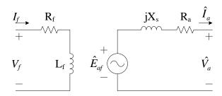
Figure 1: Per-phase equivalent circuit for synchronous generator.
