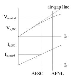
Figure 2: Typical results for open-circuit/short-circuit testing of a synchronous generator.
