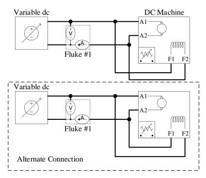
Figure 6: Connection diagram for open-circuit test
