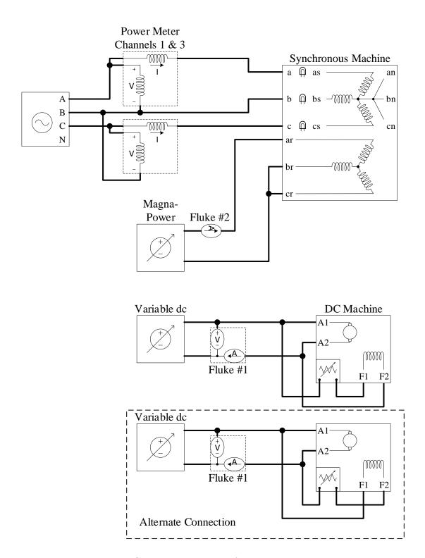
Figure 8: Connection diagram for grid-connected test
