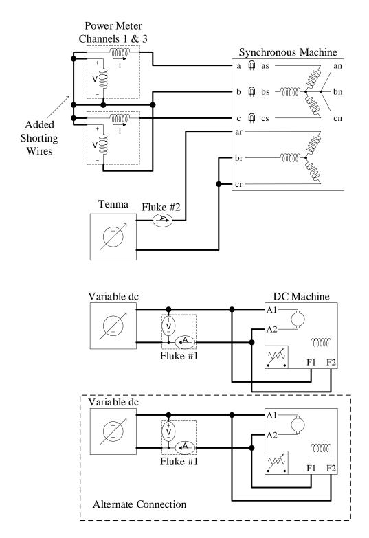
Figure 7: Connection diagram for short-circuit test
