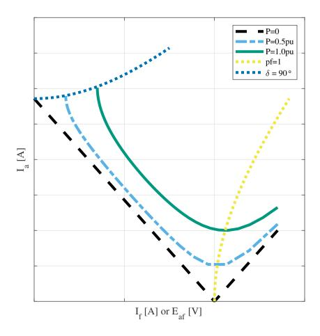
Figure 5: Typical V curves. Also indicated are the unity power factor boundary between underexcited and overexcited, and the  $\delta=90^\circ$  limit beyond which the machine cannot produce the desired power. The x axis can be field current or generated voltage.
