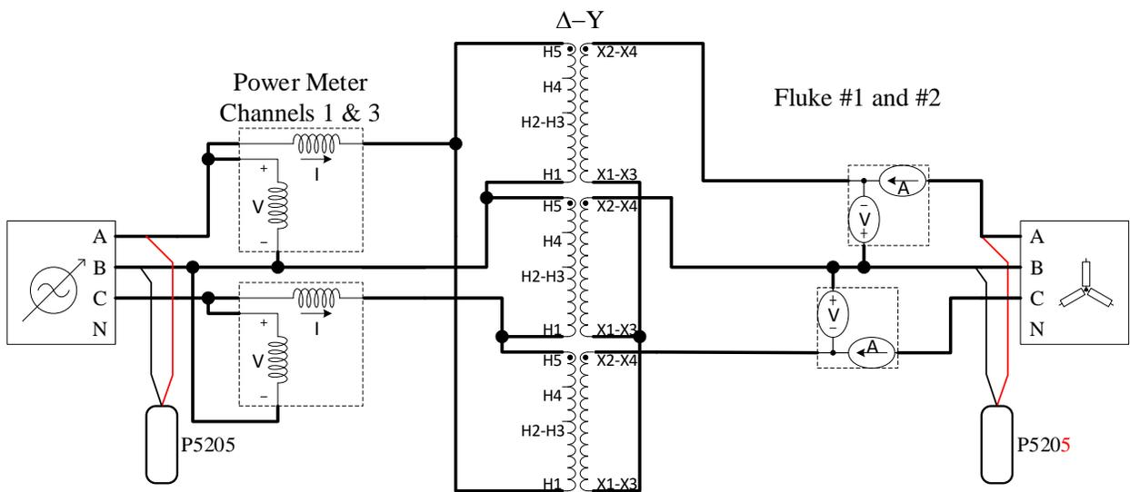
Figure 10: Experimental connections for  $\Delta - Y$  test
