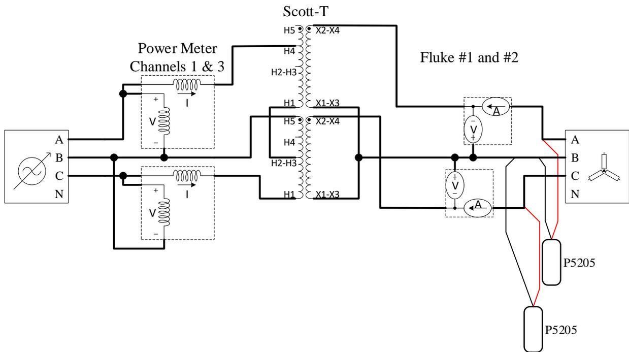
Figure 13: Experimental connections for Scott-T test
