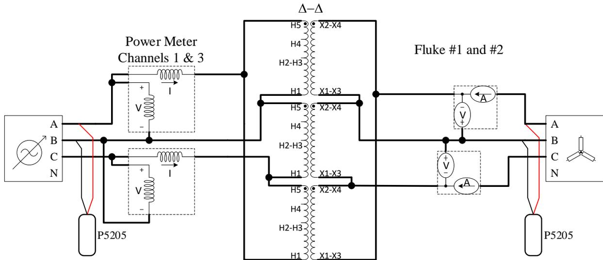
Figure 9: Experimental connections for  $\Delta - \Delta$  test
