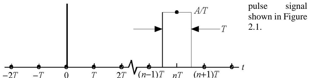
Figure 2.1 Rectangular Pulse of Area  $A$  That Approaches the Impulse  $A\delta(t - nT)$  as  $T \rightarrow 0$
