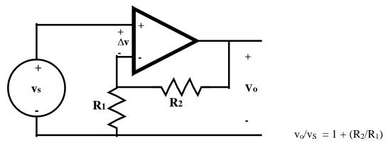
Figure 2 – Non-Inverting Op Amp Circuit
