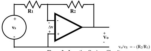
Figure 3 – Inverting Op Amp Circuit
