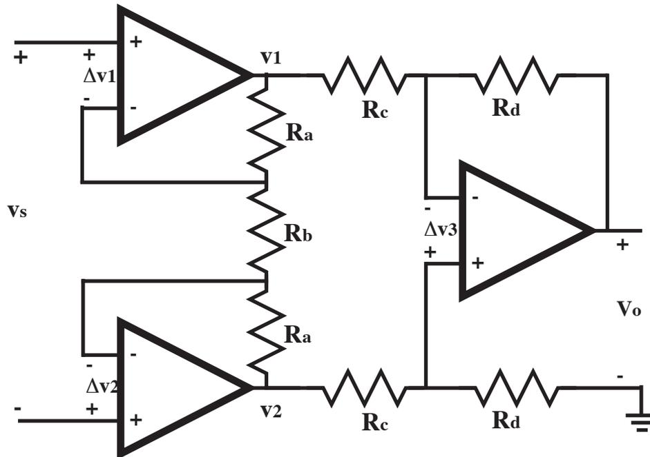
Consider each amplifier stage separately. The negative feedback drives  $\Delta v_1$ ,  $\Delta v_2$ , and  $\Delta v_3$  to zero and the OpAmp input currents are zero.
