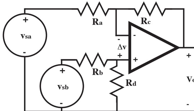
Apply superposition considering  $v_{Sa}$  and  $v_{Sb}$  separately
