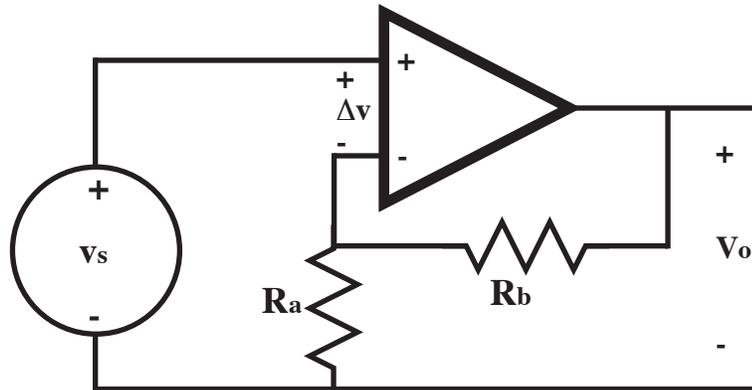
For resistors  $R_a = wR_{\text{Total}}$  and  $R_b = (1 - w)R_{\text{Total}}$  (note that  $R_a + R_b = R_{\text{Total}}$ )
