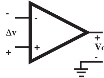
Negative Feedback – the output is connected (perhaps through various circuit elements) to the (-) terminal. Produces a stable output as  $\Delta v$  goes to zero.
