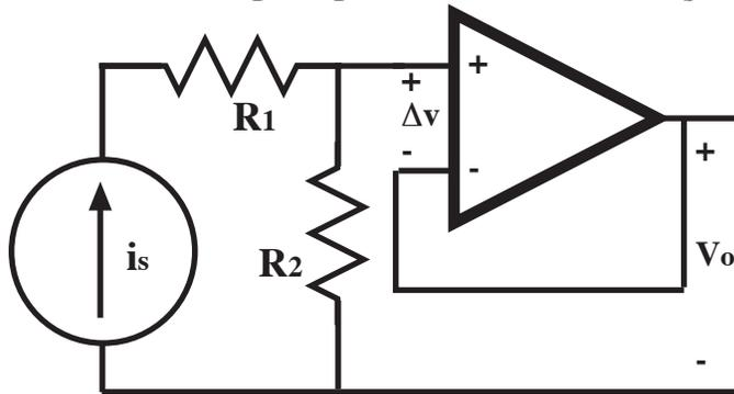
3(a) Draw the equivalent circuit in which the OpAmp is replaced with the appropriate circuit elements. Assume **ideal** input and output resistances ( $R_{out}$  and  $R_{in}$ ) and a finite gain  $A$ . (5 pts.)
