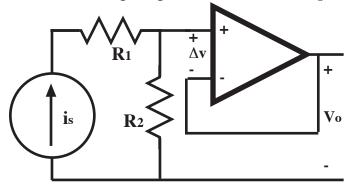
3(a) Draw the equivalent circuit in which the OpAmp is replaced with the appropriate circuit elements. Assume **ideal** input and output resistances (R<sub>out</sub> and R<sub>in</sub>) and a finite gain A. (5 pts.)
