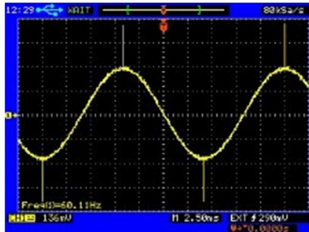
Figure 2: Sine wave with 5V DC offset as appears on oscilloscope with AC Coupling [2]
