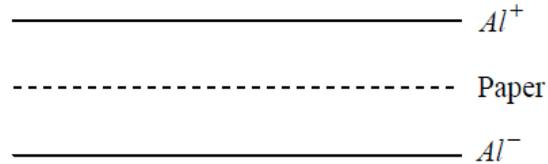
Clearly, when we roll it up we will short-circuit the plates. This can be overcome by putting in another strip of paper.
