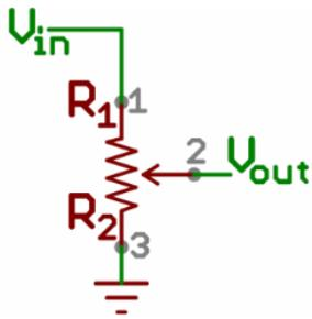
halves. Externally there are usually three pins: two pins connect to each end of the resistor, while the third connects to the pot's wiper.
