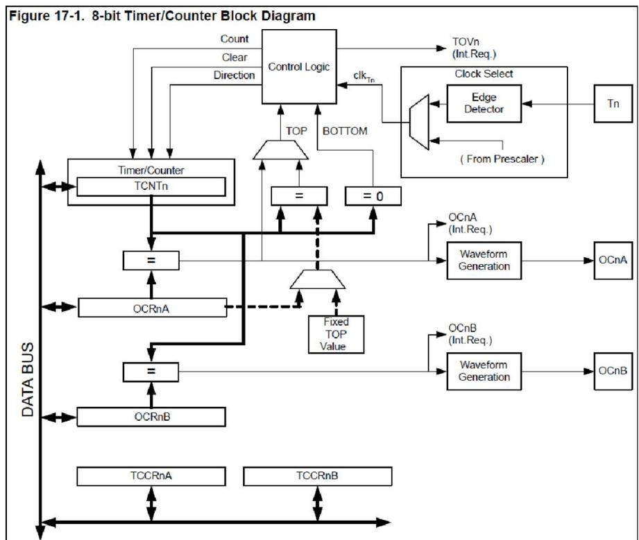
Prescaler: We already remarked that the Timer frequency can be less than or equal to the CPU clock frequency. OK, then how we decide or set the timer frequency? Here the “Prescaler” comes in! It is the method of generating the clock frequency for the TIMER from the CPU clock by dividing it with a suitable number.
