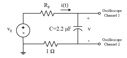
Figure 1: Circuit diagram for procedure step 3 [1]
