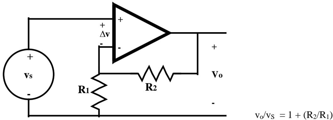
**Figure 2 – Non-Inverting Op Amp Circuit**
