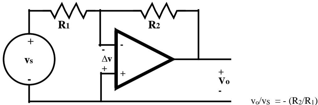
**Figure 3 – Inverting Op Amp Circuit**
