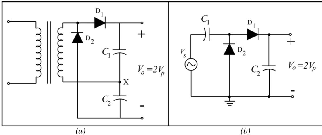
Figure 4: Two Forms of the Voltage Doubler.
