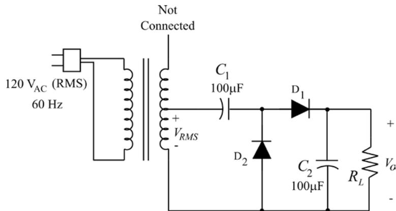
Figure 7. A half-wave voltage doubler test circuit.
