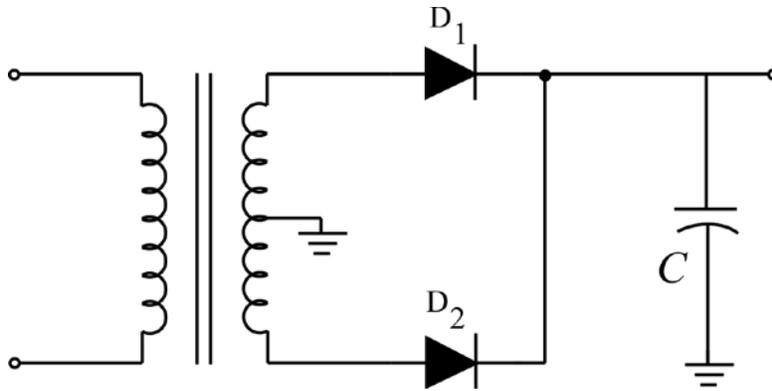
Figure 2: The Classical Full-Wave Rectifier with Capacitive Filtering.
