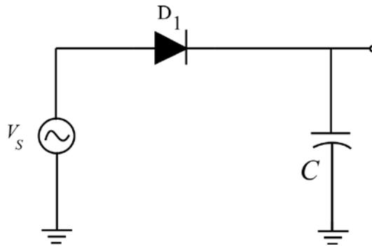
Figure 1: The Half-Wave Rectifier with Capacitive Filtering.
