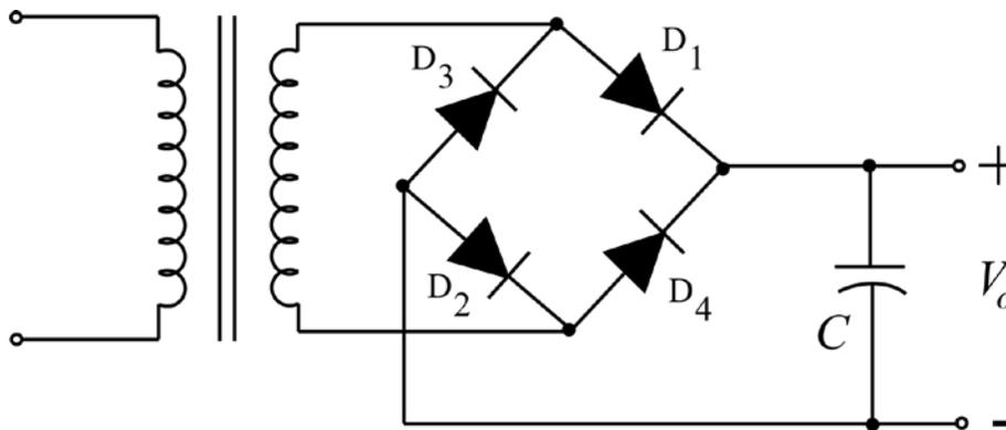
Figure 3: The Full-Wave Bridge rectifier with Capacitive Filtering.
