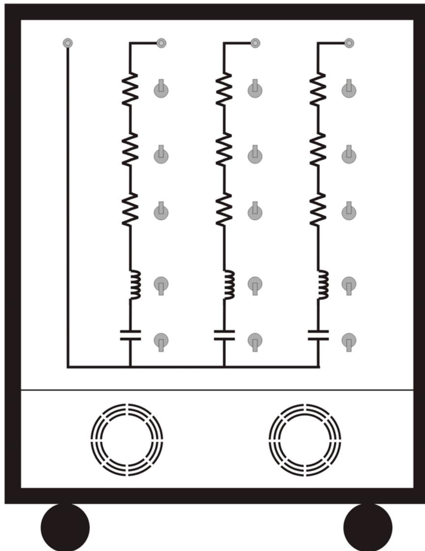
Figure 2. Load box panel.
