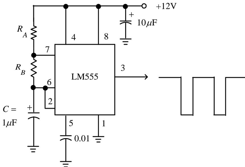
4. Power up the circuit and observe the output. How close is your waveform to your calculated parameters?
