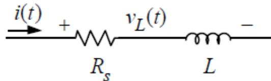
$$v_L(t) = i(t)R_s + L \frac{di}{dt} \quad (2)$$
