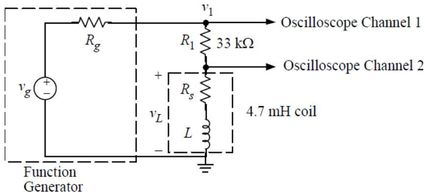
2. Set the oscilloscope triggering to positive slope, and channel 1. Set the vertical mode to dual trace. Set the signal generator for a sinusoidal output of 1 kHz. Adjust the output level of the signal generator for 20 Vpp, with a zero offset. Adjust the trigger level for a stable display. Change the volts/div for channel 2 so that the peak-to-peak amplitude of the trace for channel 2 is about 2
