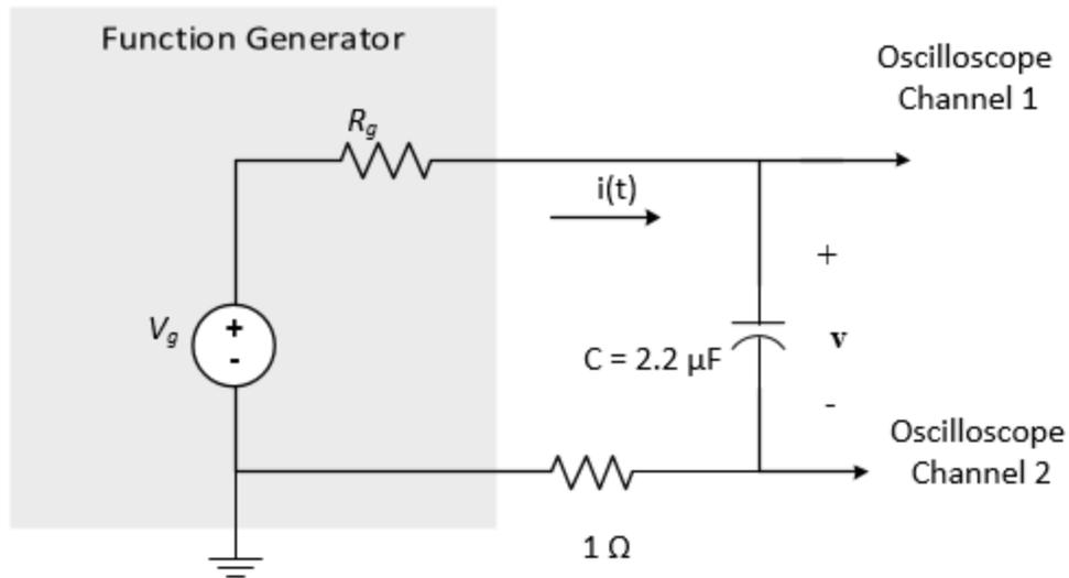
1. **Sine wave:** Turn off the math button. Set the time base to  $200 \mu\text{s}/\text{div}$ . Change the signal generator to produce a sine wave but leave the amplitude, offset, frequency, etc. controls alone.
