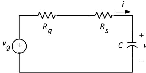
where  $v_g$  is the Thévenin equivalent voltage of the function generator. The first order differential equation relating the voltage across the capacitor,  $v$ , to the source voltage,  $v_g$ , is:
