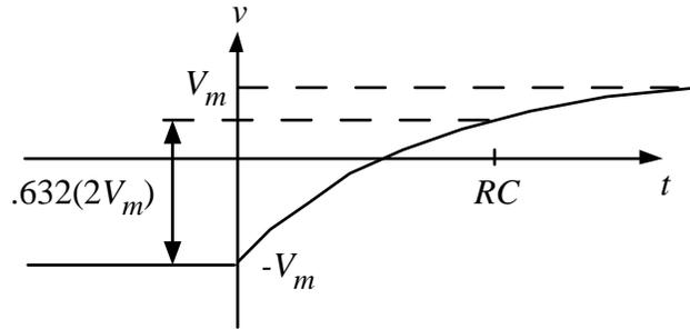
At the time equal to  $RC$  (which is called the *time constant*), the exponent has a value of  $-1$ . So, the value of the response at this point is,
